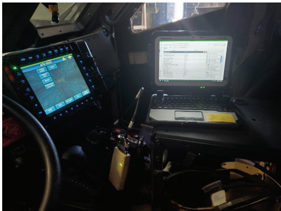
An Electronic Maintenance Support System running diagnostics on a Joint Light Tactical Vehicle. (Courtesy of MCSC.)
