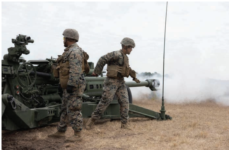
Cpl Erick Leon, right, a Queens, NY, native and a field artillery cannoneer with 1/10 Mar, fires an M777 towed 155 mm howitzer during field training on Camp Lejeune, NC. (Photo by LCpl Jonathan Rodriguez Pastrana.)
