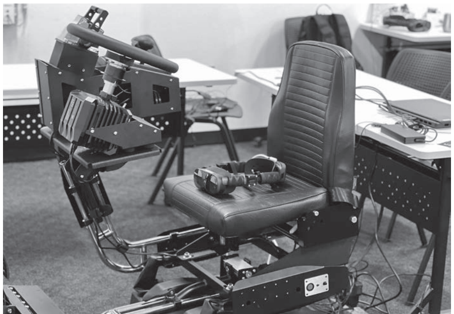
Driver training system consisting of VR goggles, mixed reality steering wheel, gear shift, marine propulsion controls, and a two-direction of freedom chair. (Photo by VR Training.)
