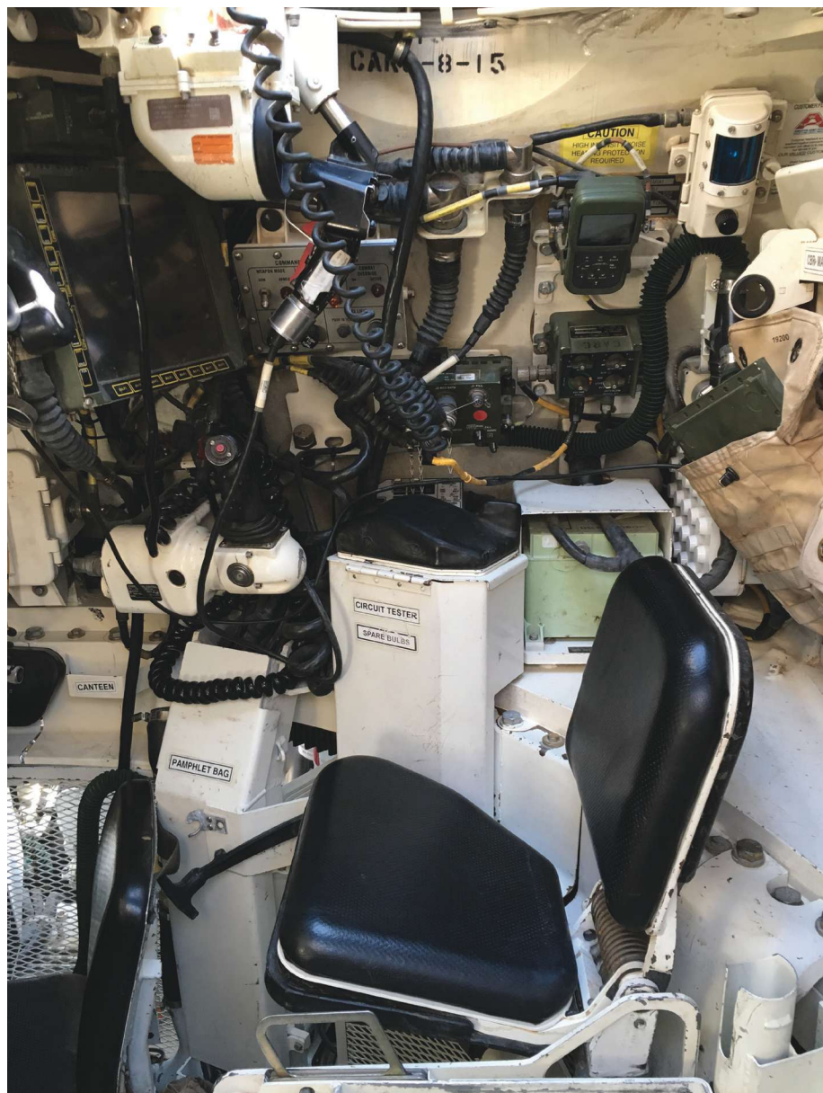
Originally upgraded in 1985 to be capable of operating in an EW denied/degraded environment against the Soviets, the M1A1 tank accumulated several C2 upgrades in the last nineteen years before it was divested in 2020. Pictured here is the author’s tank commander’s station and all the cables that supported modern C2 upgrades like the AN/PSN-13 DAGR and FBCB2 “Blue Force Tracker.” These modern C2 systems made the M1A1 an EW liability for a peer threat. (Photo from the author.)
