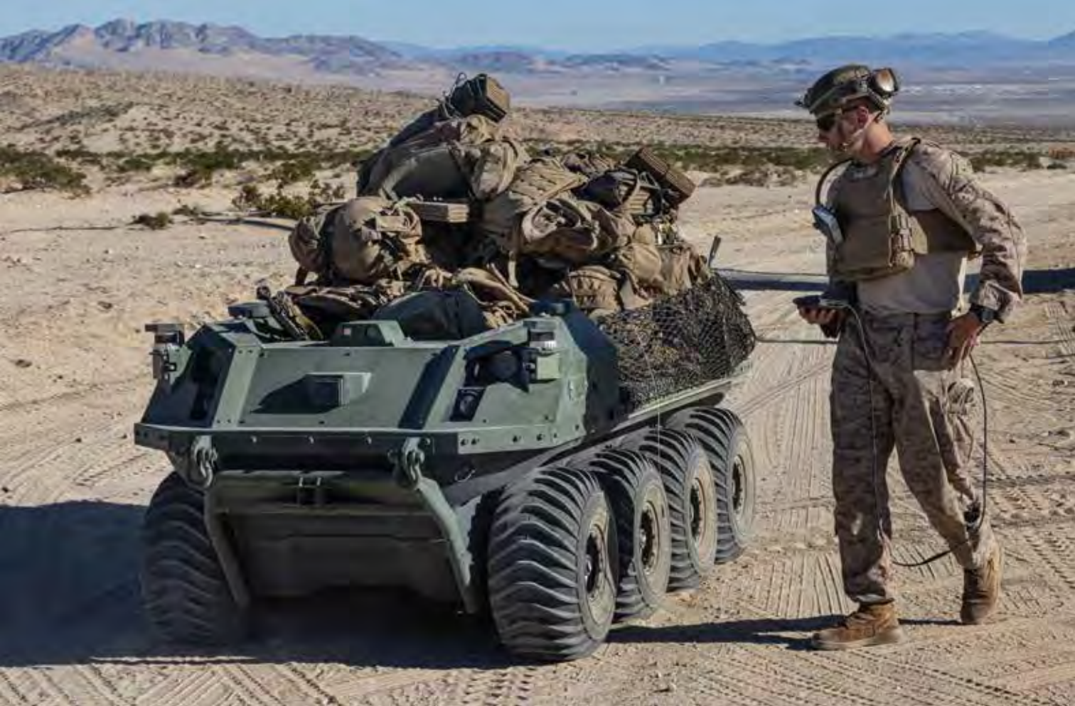
LCpl Hayden Frank, an infantry Marine with 3rd Bn, 4th Marines, 7th Marine Regiment (Rein), transports gear with a “Mission Master” unmanned ground vehicle during Exercise Apollo Shield on Oct. 11, 2023. The Mission Master is an autonomous vehicle that increases logistical flexibility. (Photo by Cpl Jonathan Willcox, USMC)
