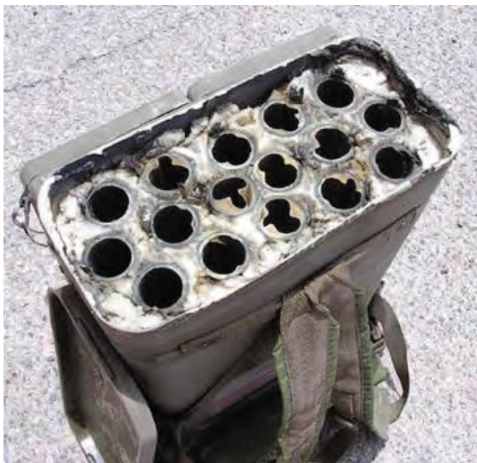
Above left: The E8 Tactical CS Launcher, which was carried as a backpack, could send 16 CS projectiles toward a target and was used during the assault from An Tan Ridge.
