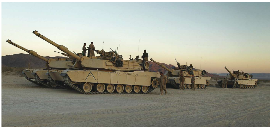
The decision made was to have 7 road wheels on the Abrams M1 A1 tank. (Photo by Cpl Sarah Dietz.)
