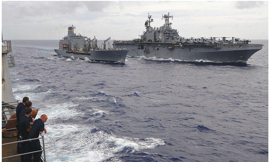
Ships in the Nassau (LPH 4) Amphibious Ready Group conducting an underway replenishment operation. (Photo by Mass Communication Specialist 2nd Class Jason R. Zalasky.)
